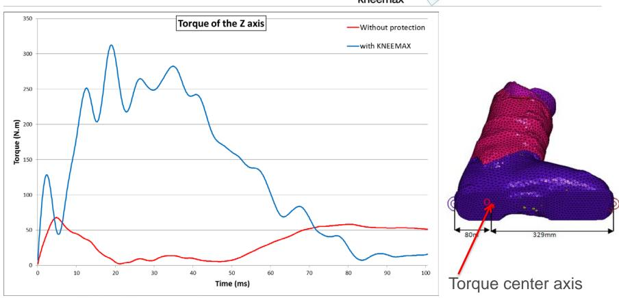
Solid blue line KNEEMAX® shows a growth of the release's torque of the ski bindings during a non physiological movement.
