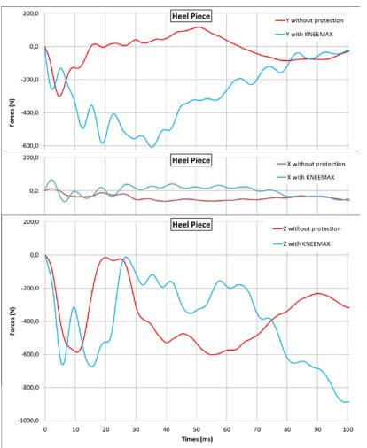
KNEEMAX® improves the efficiency of the ski bindings by creating a stronger signal (according to Y axis) from the lower limb to the ski binding.
